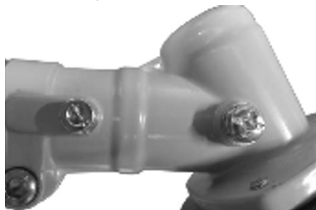
Pic. 21 Bolt holes for gearbox lubrication
