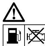
Switch the engine off and allow to cool before refuelling the generator. Fuel is extremely flammable and under certain conditions can be explosive. Only refuel the generator in well ventilated areas ensuring that naked lights, sparks and cigarettes are not present. Any spillage of fuel should be immediately cleaned up.
